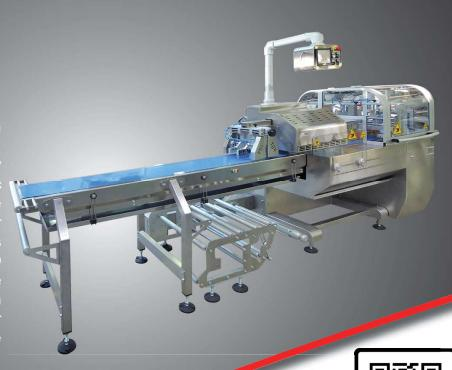
Performances up to 25 bpm intermittent / 80 bpm box motion version Stainless steel structure
